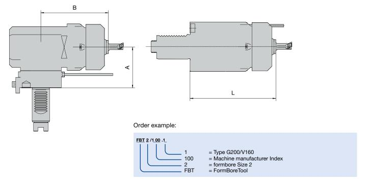
A, B, L = Dependent on the machine interface
